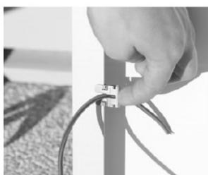
❶ Position grounding clip with electrical cable inserted in it and the bottom of the part outside the frame
