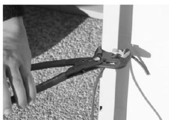
❷ Place the plier by gripping the clip with the external jaw and internal jaw set on external face of the module frame
